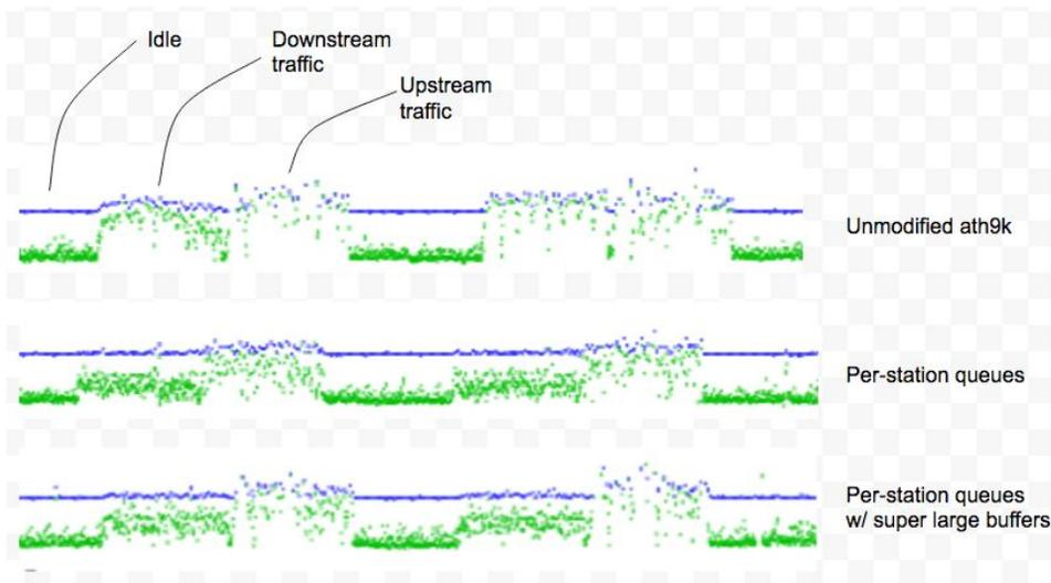
Latency effect on station A of simultaneous traffic to/from station B
